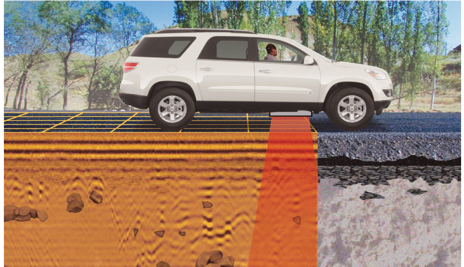
Localizing Ground-Penetrating Radar (LGPR) uses relatively stable subsurface features and their geolocation to locate the vehicle even in adverse weather conditions.
